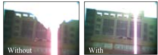
Figure 5: Image of building without (left) and with (right) DSF within an external module.
